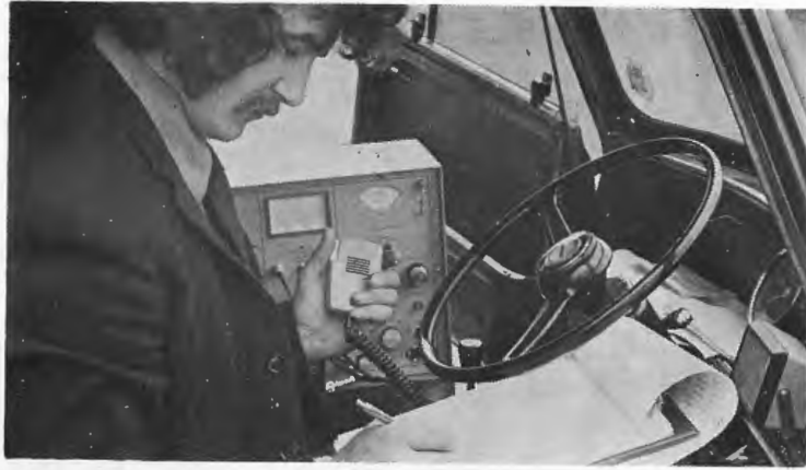
Right, Dave Watts ( Industrial Staff Trainee ), checking the performance of a mobile unit following installation.
